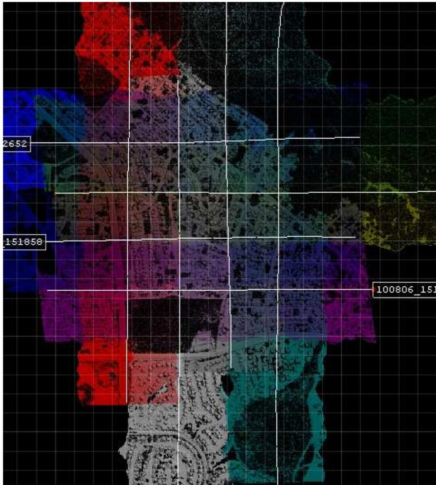
**Figure 3.** Boresite Flight Lines and Trajectory Visualization.
