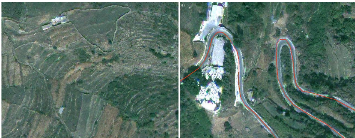
Figure 4. Komiaki region (650 m elevation) in the island of Naxos in R,G,B channels orthorectified in full spatial resolution. Left: Detail showing the stony walls and the terraces. Right: Detail showing the matching between the orthorectified image and the vectorized 1983 map road. Satellite image of GeoEye-1 of 0.5 meter spatial resolution pan sharpened in four 11-bit channels dated October 23, 2009.
