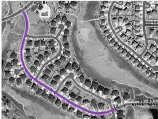
Figure 18. RoadTracker automatically finds the road between the start and end point.
