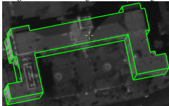
Figure 12. The building after the height is estimated and accepted.
