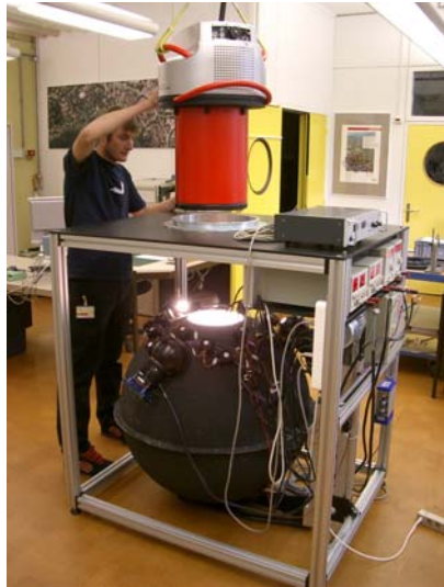
Figure 2. Radiometric calibration facility (left) and calibration procedure for the integrating sphere (right).
