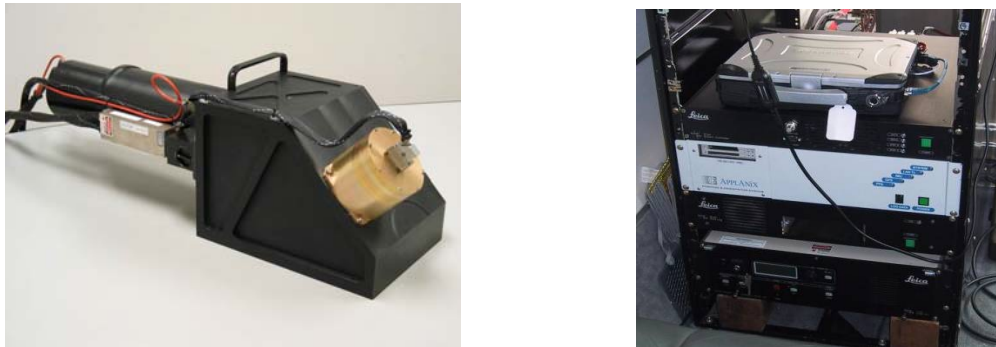
Figure 2. Complete lidar profiler system with sensor (left) and rack (right).
