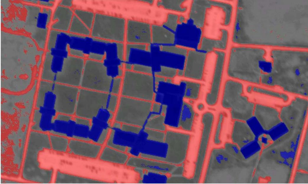
**Figure 4.** Thermal Survey for Engineering and Environmental Analysis – Classified thermal tile with 50 cm GSD.
