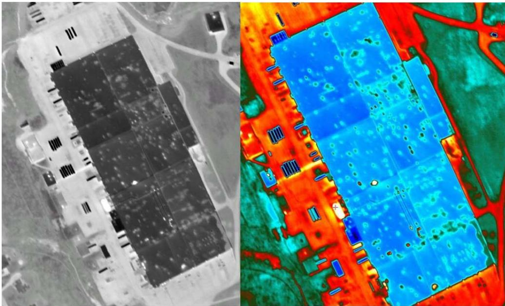
**Figure 2.** Thermal survey for roof inspection, Left: Panchromatic thermal image, Right: Colorized thermal image.
