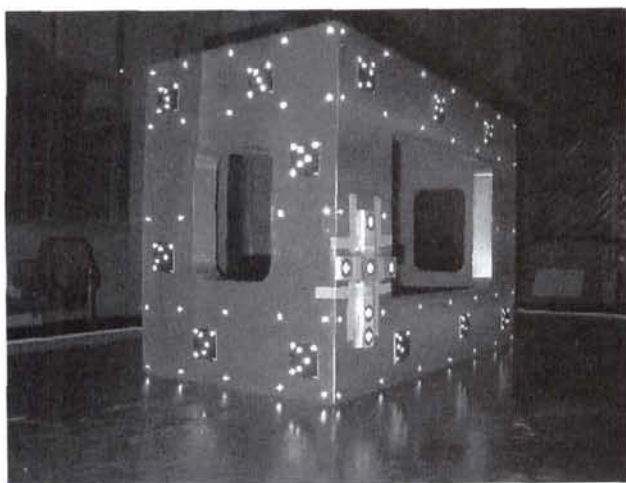
Figure 8. Test box structure showing EO device, CTs, and MTs.
