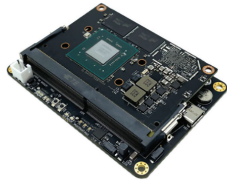
Figure 4. PixC4 with Nvidia Jetson Xavier NX.
