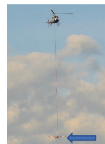
Figure 31. Helicopter with towed "bird" with MAG RAD sensors. Source: Sander Geophysics Ltd.
