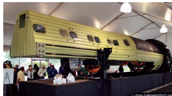
Figure 16. Now on display at the National Museum of the United States Air Force near Dayton, OH, the KH-9 Hexagon reconnaissance satellite was declassified on 9/17/2011. At 60-foot length and weighing 15 tons at launch, 19 KH-9 satellites were launched between 1971 and 1986. Panoramic images were film, not digital. Personal image.
