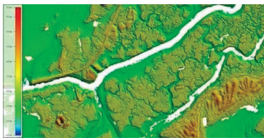
Figure 24. Topobathy lidar mapped portions of the river, but not the deeper tannic waters with mucky bottom. Image source: Dewberry.
