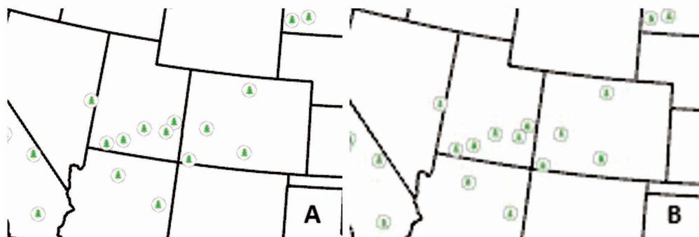
Figure 1. A portion of a map showing National Parks in the western U.S. Map A was scanned at 300 DPI while Map B was scanned at 50 DPI.
