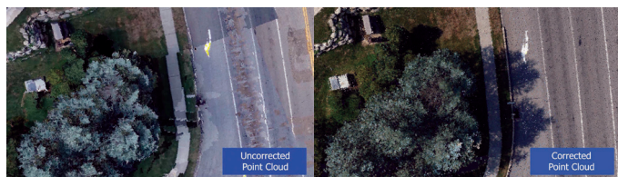
Uncorrected versus corrected lidar point cloud models
