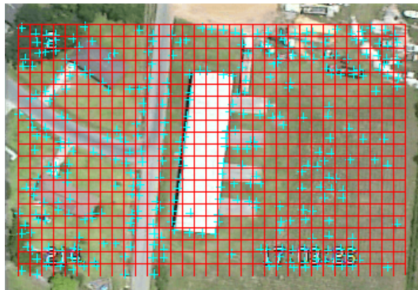
Figure 3. Method for extracting IP within grid and the perdition of the conjugate point (blue cross).
