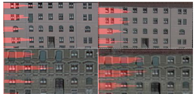
Figure 4: Two examples for floor detection using edge histograms. The oblique images are to the left.
