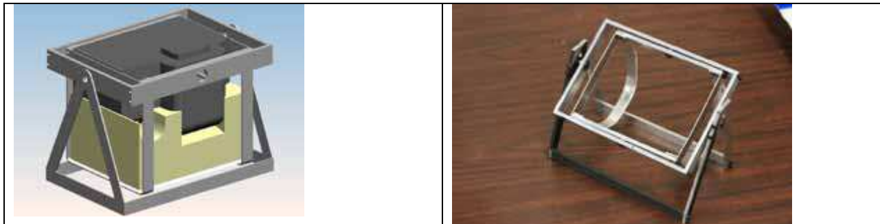
Figure 4. Camera mounts design and implementation.
