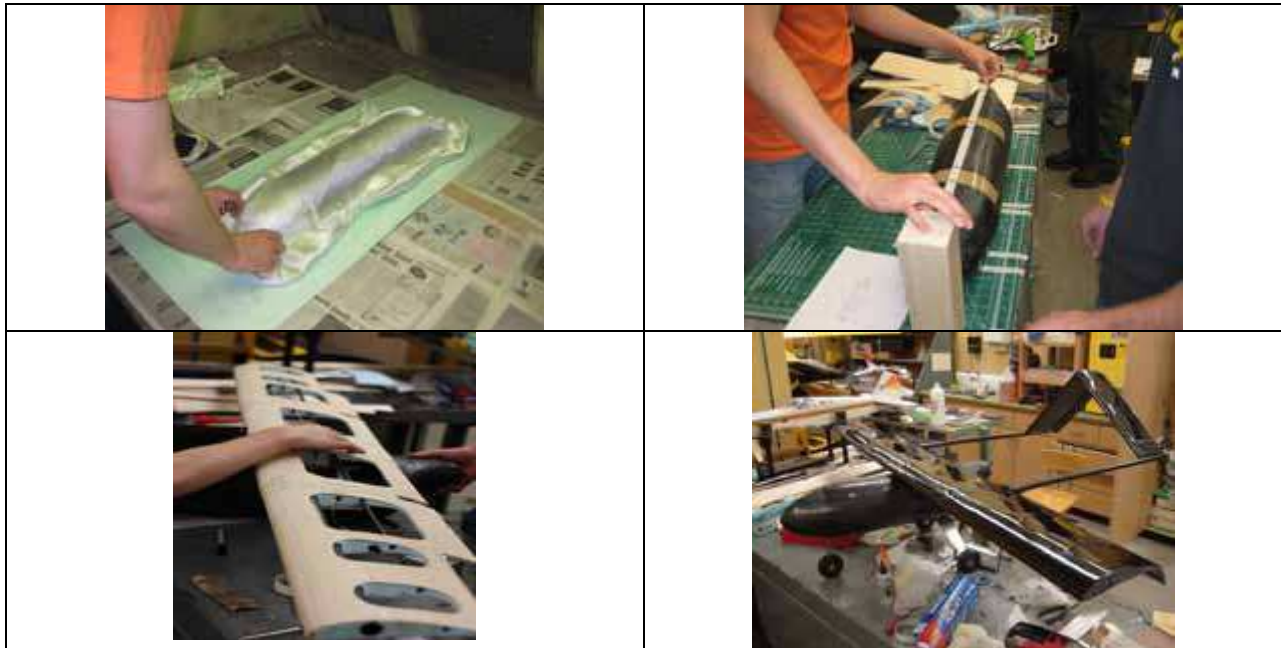
Figure 3. Airframe and fuselage fabrication.
