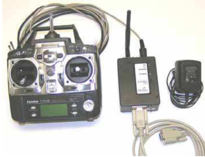
Figure 7. PSUAV ground control system.
