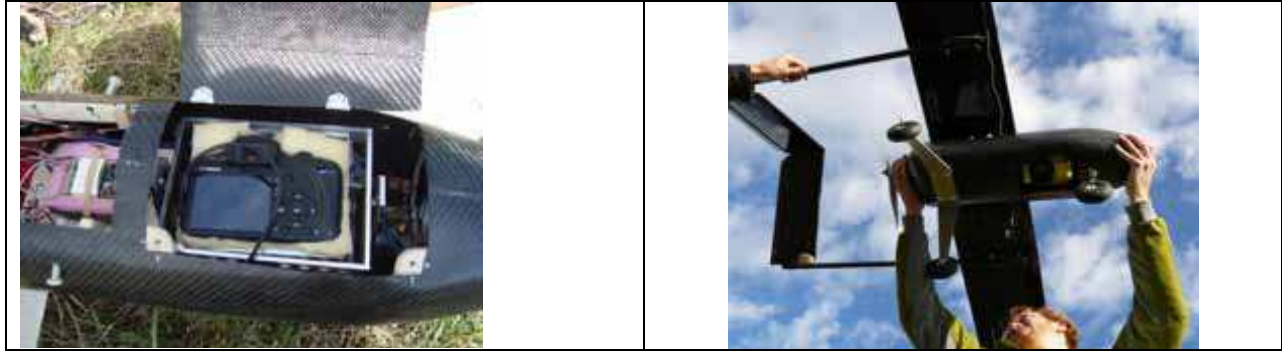
Figure 5. Camera installed into PSUAV mount during test flight.
