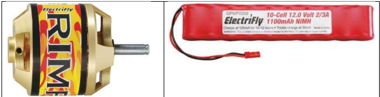
Figure 2. Electrical engine and batteries used for PSUAV.
