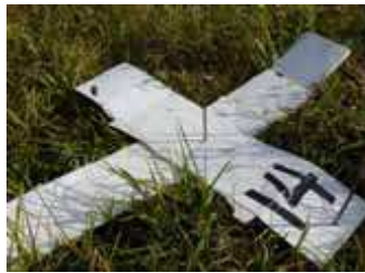
Figure 10. Photogrammetric target is installed on the ground.
