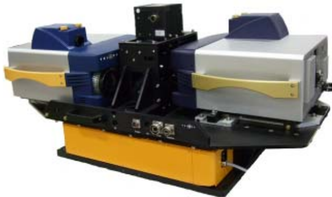
Figure 5. Illustration of the airborne configuration with two Hyper-Cams.
