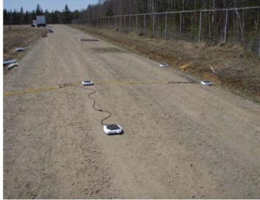
Figure 6. Ensemble of 4 hotplates used to test pixel size definition.
