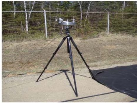
Figure 9. Weather station mounted at the experimental site near the gas plume generator.
