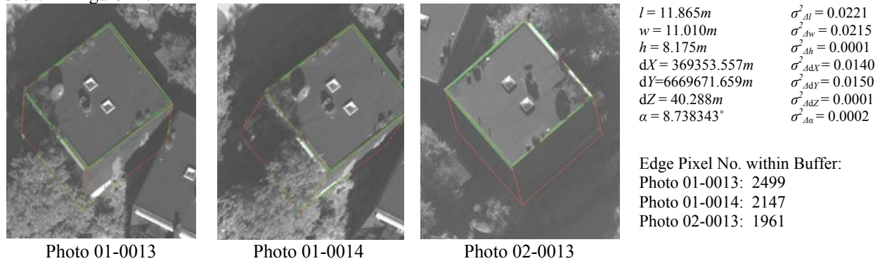
Figure 13. The box primitive model achieves optimal fit after 20 iterations by using both aerial photos and LiDAR data. (Initial horizontal buffer size: 0.5mm )
