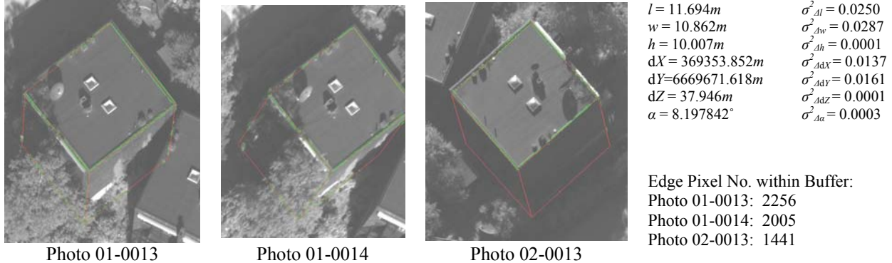
Figure 12. The box primitive model achieves optimal fit after 5 iterations with constrained dZ .
