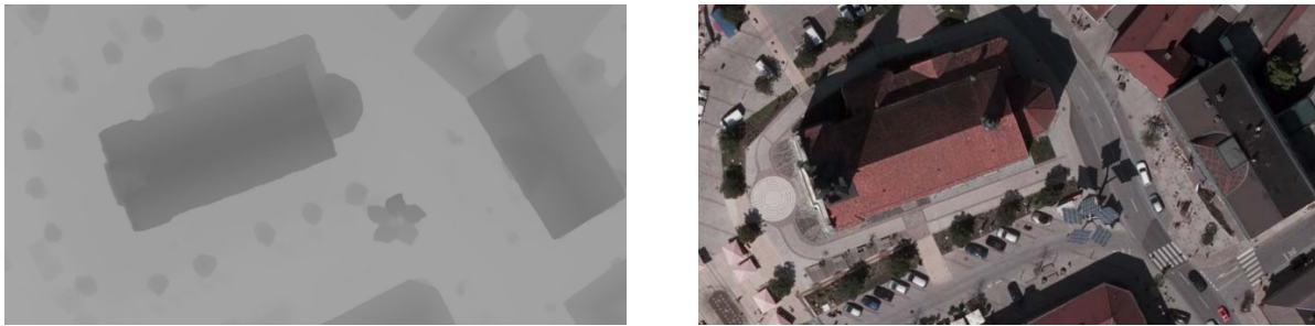
Figure 10. High resolution DSM by dense matching of UltraCamL images (left) and 10cm GSD true-ortho image (right).
