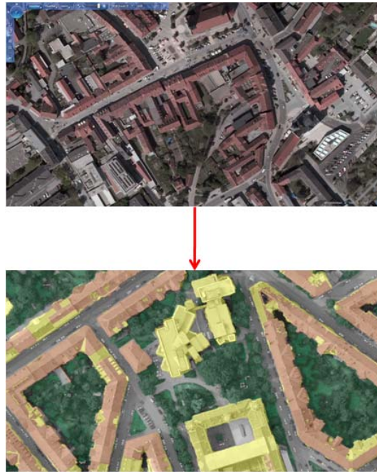
Figure 11. Classification map generated out of an UltraCamL by computer vision.
