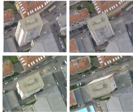
Figure 7. Highly redundant data set. One object is visible in up to 15 images due to the specific flight pattern.
