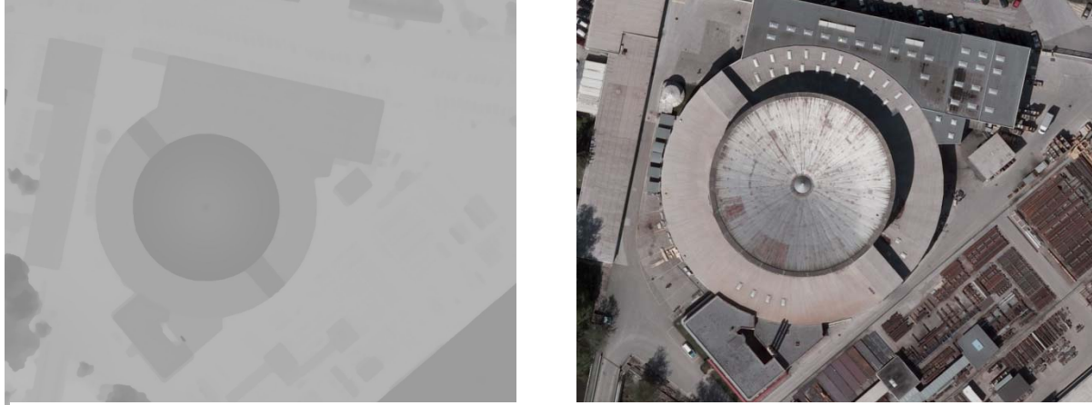
Figure 9. High resolution DSM by dense matching of UltraCamL images (left) and 10cm GSD true-ortho image (right).
