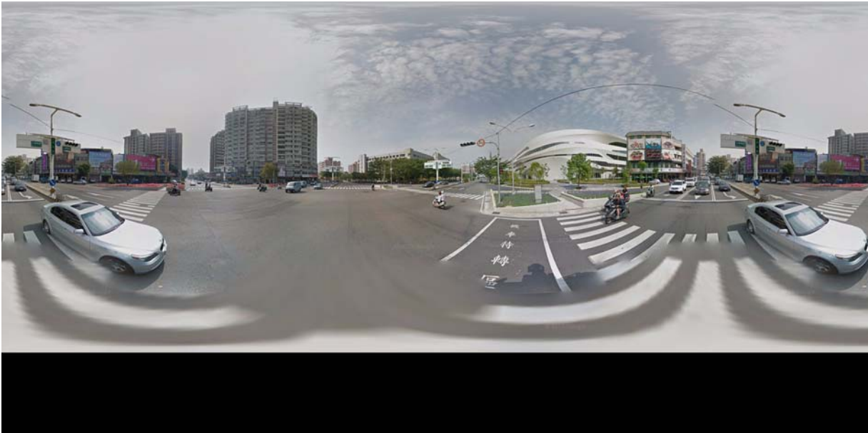
(a) Original tiled GSV panorama with horizontal overlapping, distortion, ghost, and empty block (size: 2048x1024)
