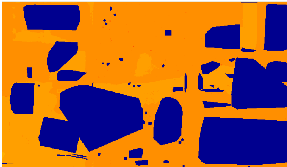
Fig. 07. Elevation map of ground points outside convex-hull (Orange), convex hulls (Blue)
