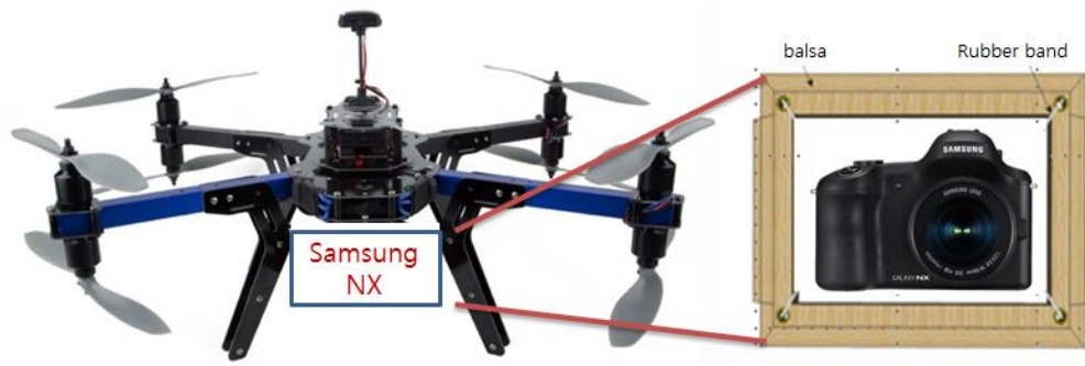
Figure 2. A dustproof device designed in order to reduce high frequency vibration from UAV(X-8 Copter)
