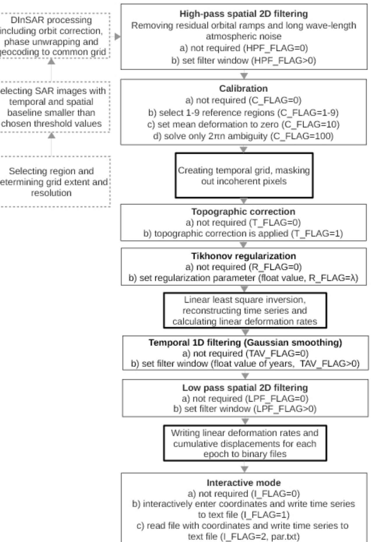
Multidimensional Small Baseline Subset (MSBAS), Samsonov and d'Oreye, 2011, Samsonov et al., 2014) methodology combines ascending and descending InSAR data and produces horizontal and vertical deformation time series and mean rates.
