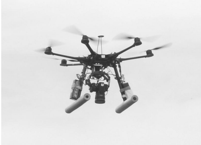
Figure 4. DJI S800 "Spreading Wings" hexacopter in its overflight carrying a modified Canon EOS Rebel T4i DSLR camera.
