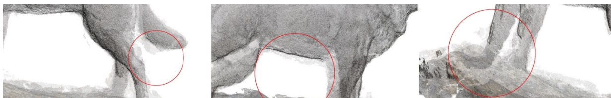
Figure 8. Blunder or wrong points in the achieved point clouds (red circle)
