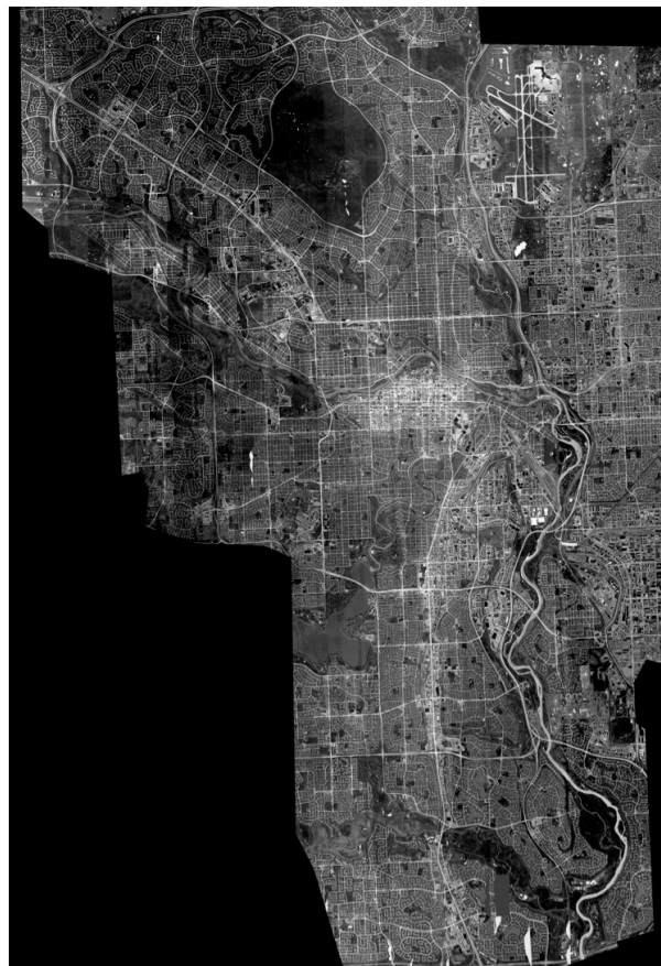
Figure 1: TABI-1800 temperature map of Calgary. (N is up, 40km X 27km, 0.5m/pixel)
