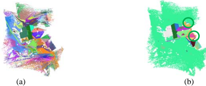
Figure 13. Dataset3: Adaptively Down-sampled dataset – Planar segments (a) before and (b) after Quality Control
