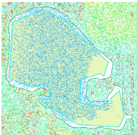
Figure 16: Polygon feature drawn manually inside the hydro break line to calculate water surface elevation
