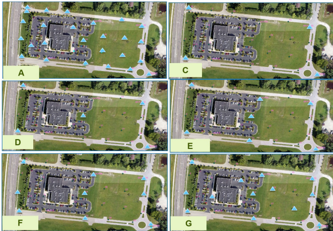
Figure 5: Ground controls evaluation scenarios for Case I. (The blue triangles represent control points used in the processing.)
