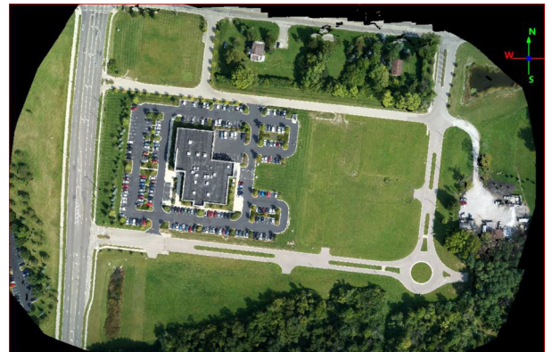
Figure 6: Colorized point clouds derived from the UAS-based imagery.
