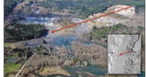
Figure 1. Oblique aerial view and smaller-scale lidar image (inset) of the Oso, Washington, landslide of March 22, 2014. Red arrows point to upper edge of scarp and show direction of material flow. Photograph taken on April 1, 2014, by Mark Reed (USGS). Lidar image derived from 3DEP data collected by the Washington Department of Transportation on March 24, 2014.
