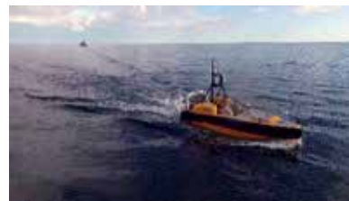
Figure 28. With the mothership in the background, such USVs are ideal for shallow-water surveys using a variety of SBES or MBES sensors. Source: TerraSond.
