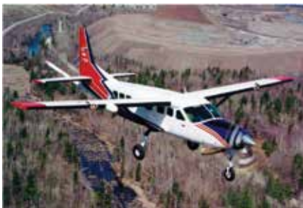
Figure 29. Fixed-wing geophysics aircraft with stinger in the rear. Image source: Sander Geophysics Ltd.
