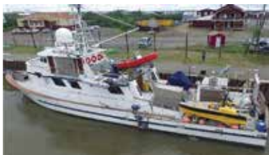
Figure 27. Larger vessel (mothership) used for traditional MBES surveys in deeper water and CW5 USV (yellow) used for shallow-water surveys. Source: TerraSond.
