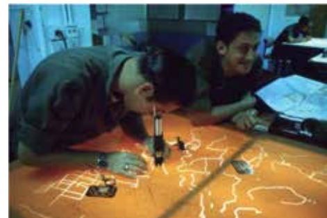
Figure 6. Although these scribed lines are thick for visualization purposes, most scribed lines are a small fraction of a mm thick and require a steady hand scribing beneath a microscope. Personal image.
