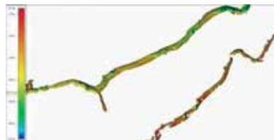
Figure 25. Multibeam sonar mapped the deeper parts of the river not mapped with topobathy lidar. Image source: Dewberry.
