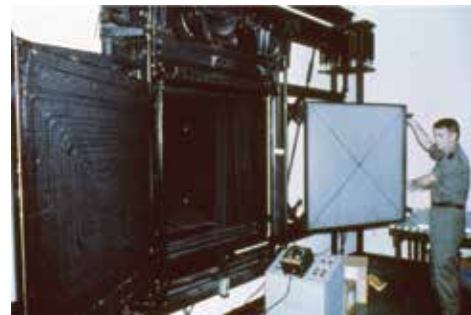
Figure 5. Walk-in mapping camera used by my topographic engineer battalion in Hawaii to produce the L653 series of topographic maps for U.S. Forces, Korea. Personal image.
