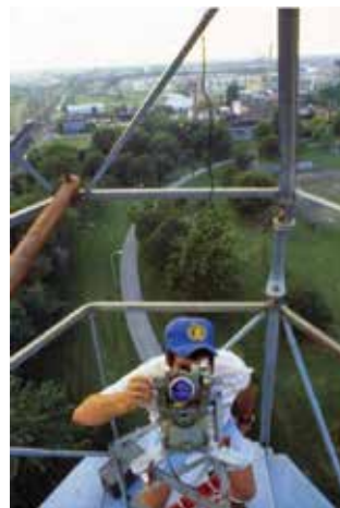
Figure 11. T-3 triangulation measurement from a USC&GS Bilby tower. NOAA Photo Library.
