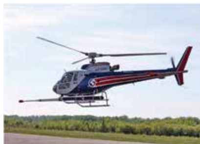
Figure 30. Rotary-wing geophysics aircraft with stinger in the front. Image source: Sander Geophysics Ltd.
