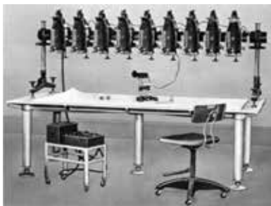
Figure 17. Multiplex projectors where I first learned to perform stereo photogrammetric map compilation in the Army. This was the easiest to visualize how aerial geometry was replicated at reduced scale to perform relative and absolute orientation. Source: US Army.
