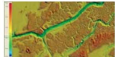
Figure 26. By merging the two datasets, the entire topographic and bathymetric surface was mapped seamlessly. Image source: Dewberry.
