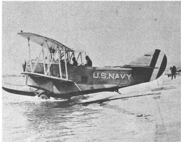
Fig. 5. Early Loening amphibian used for many years for photographic mapping by the Navy.
