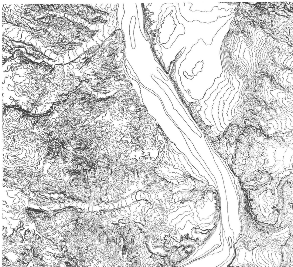
Fig. 10. Sheet of Boulder Reservoir Survey made with Stereoplanigraph (reduced to 1/3 actual size in reproduction. Original on scale of 1:12,000 with contour interval of 10 feet).
