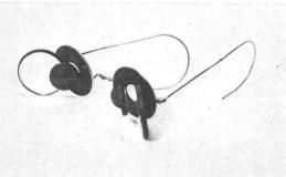
Koningh, Photogrammetric Instrument-makers in Arnhem (Holland), have constructed a pair of stereoscopical eyeglasses. With this stereoscope the maximum separation of the prints is such that even prints of  $30 \times 30$  cm. (11.8×11.8 in.) size can be seen stereoscopically at one setting.
