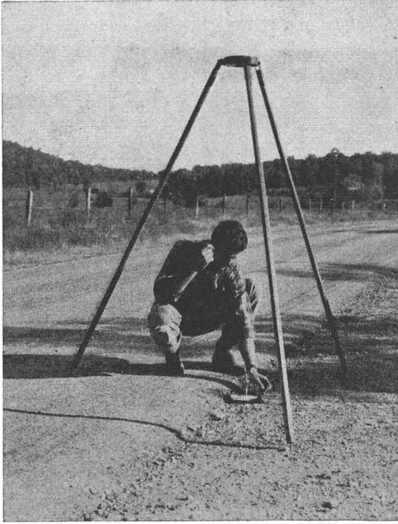
Alignment of mirror under collimator head by the use of a plumb bob.
