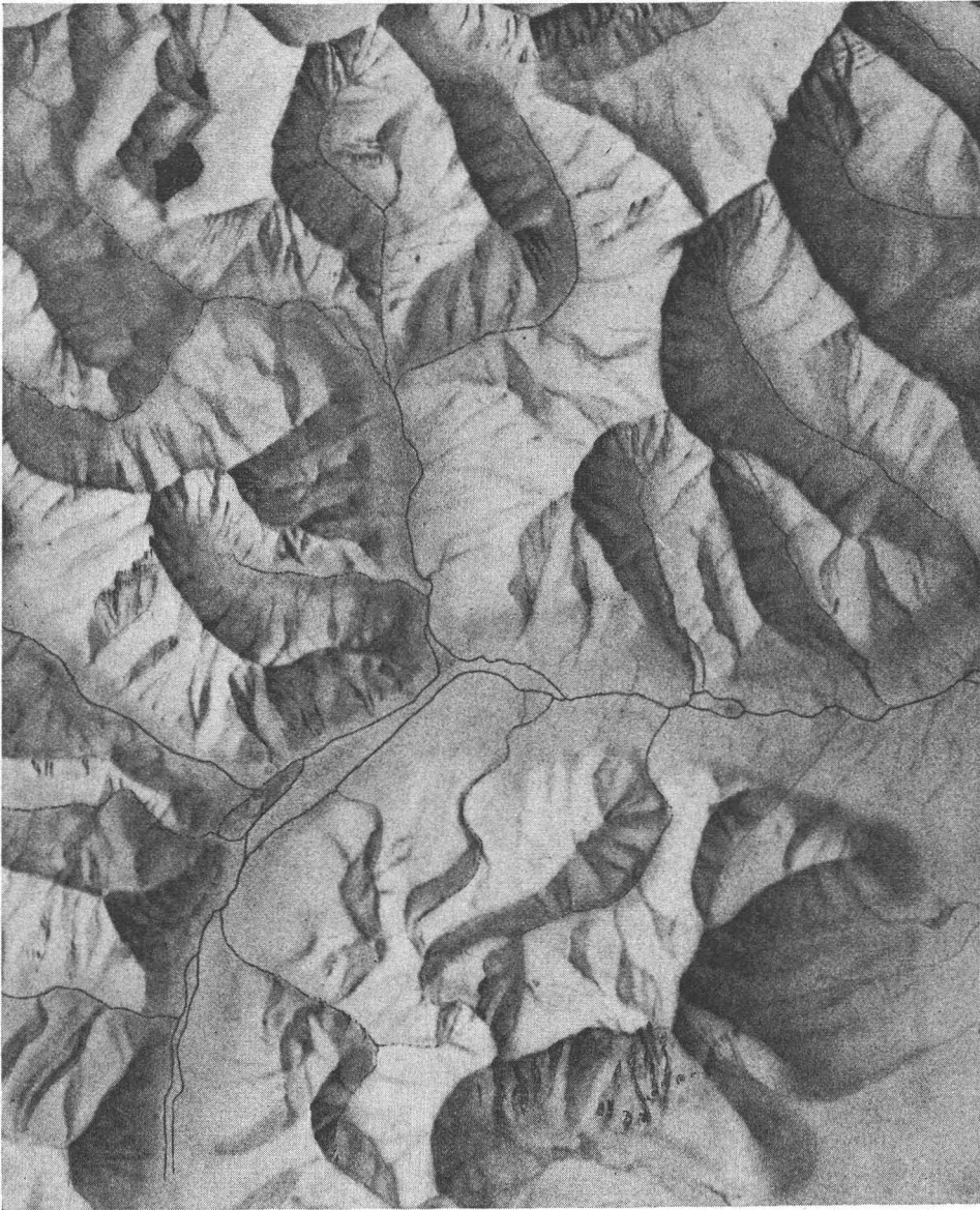
FIG. 1. Sample shaded plate made on planimetric base, from high oblique shown in Figure 2.
