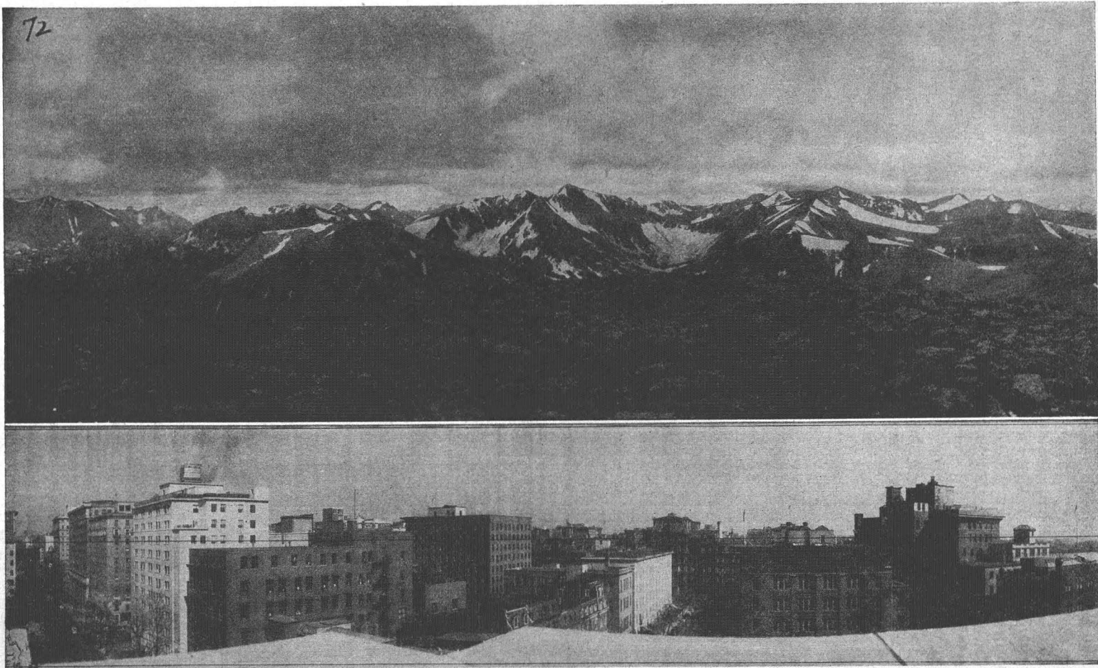
FIG. 2. Photos taken with old and new type cameras (about one-third contact print scale, covering 125^\circ of horizon). Lower print is about one-third of entire exposure.
