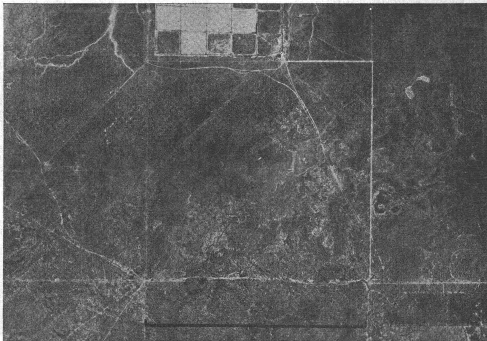
FIG. 28. Soil pattern of sands and clays under arid climate (3 to 10 in. rainfall) near the central portion of a filled valley. Fine sands have the lighter color, are slightly higher in elevation, and bear the channel marks of the outwash from the mountains. The clay settles out as lacustrine material in relatively quiet waters giving a contrasting dark tone compared to the sand. These areas may be under water for short periods each year.
