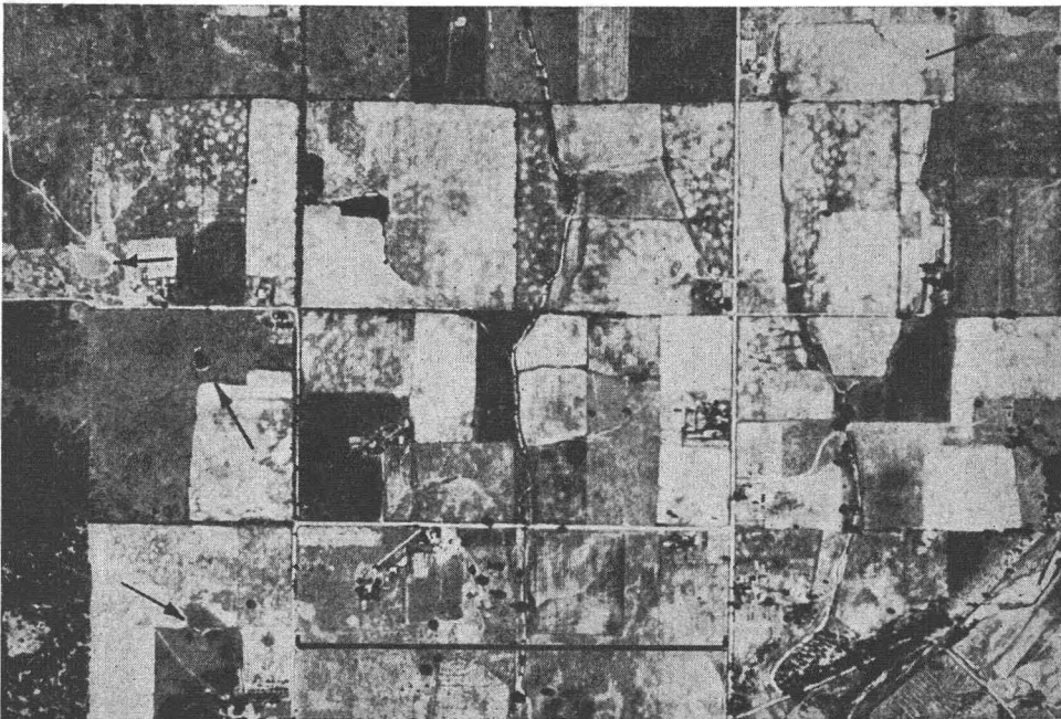
FIG. 8. Illustrations of a soil pattern in a cherty limestone area. Sinkholes (arrows) indicate limestone. The white speckled pattern is related to the chert and indicates a particularly difficult compaction problem. Close observation of cut slopes and detailed ground inspection are necessary to distinguish this condition when on general reconnaissance survey.
