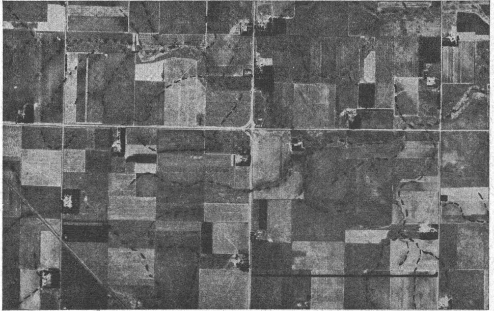
FIG. 24. An air view of a plastic silty clay soil and a tracing of the surface drainage pattern. Note the transition from drainage ways to a dark color pattern. Compare the drainage pattern on these Nos. 10 and 11 soils with the sand (No. 2) pattern in Fig. 23.
