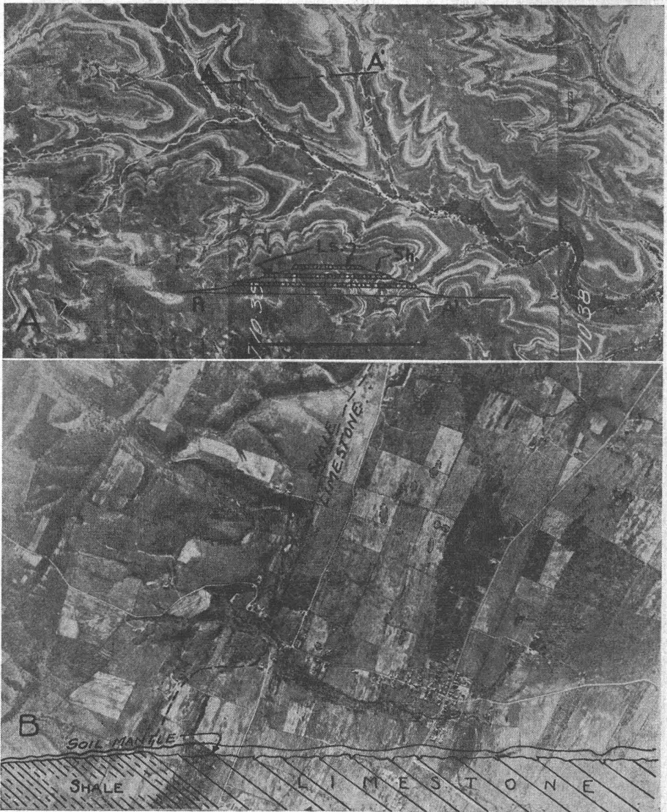
FIG. 13. A. Aerial view of nearly horizontal beds of limestone and shale. Geologic erosion has cut through a series of these strata forming a contour-like pattern. In this relatively dry climate the limestone (white) outcrops to form comparatively steep slopes while the soft shale (dark) assumes low, gentle slopes. Sketch on section A-A' illustrates formation. B. Down-dipping beds of shale and limestone form the pattern shown. Shallow impervious soils form on the shale while deep soils mantle the limestone. Note the abrupt change in surface drainage.
