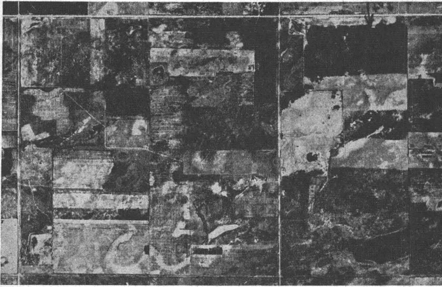
FIG. 10. A semi-granular glacial drift area in a dry climate. Lack of vegetative cover and the type of land use indicate a semi-arid condition. Semi-granular texture is indicated by lack of surface drainage. Notice the directional trend of the pattern influenced by the ice movement.
