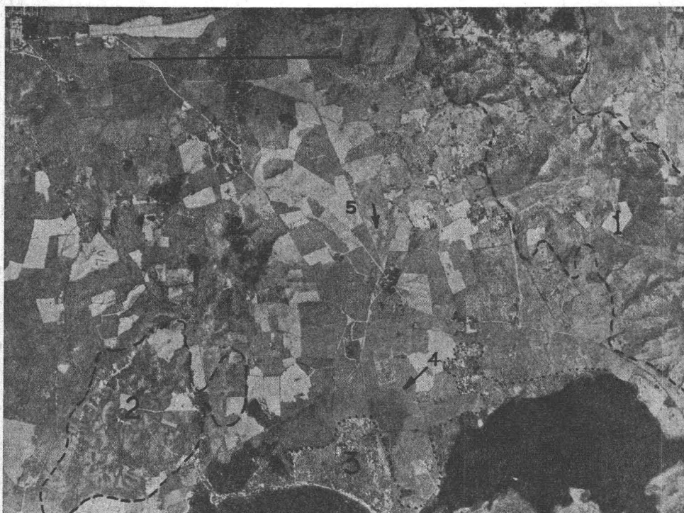
FIG. 25. A vertical photograph of an area containing a lateritic soil, 1, in which clay size soils function as porous material. Laterite may develop from any type of parent rock under conditions of high rainfall and temperature. Plastic soils developed on comparable slopes, 2, from tuffaceous rock have developed a surface drainage pattern. Sand bordering the shore line is shown in dotted outline, 3. Arrows indicate, 4, a swamp area, and 5, a color pattern indicating highly plastic soil.
