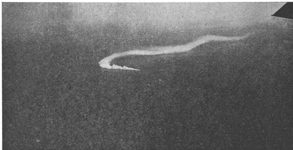
FIG. 3. Two intersecting patterns of bands, Feb. 6, 3:00 P.M., from 3900 feet altitude. Smoke laid by ship steaming on slightly curved course nearly into surface wind. Undulating tail of smoke train shows direction of upper wind and alternate zones of stable air and rising air.
