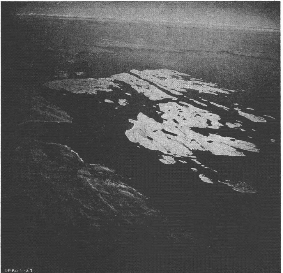
FIG. 11. Oblique photograph of islands in Frobisher Bay with K-17 camera; tilt 56.8^\circ .
