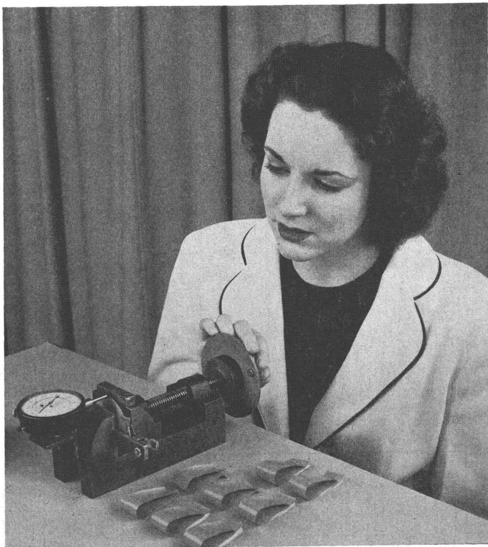
FIG. 12. Testing Safety Aerographic Film for "vise brittleness."
