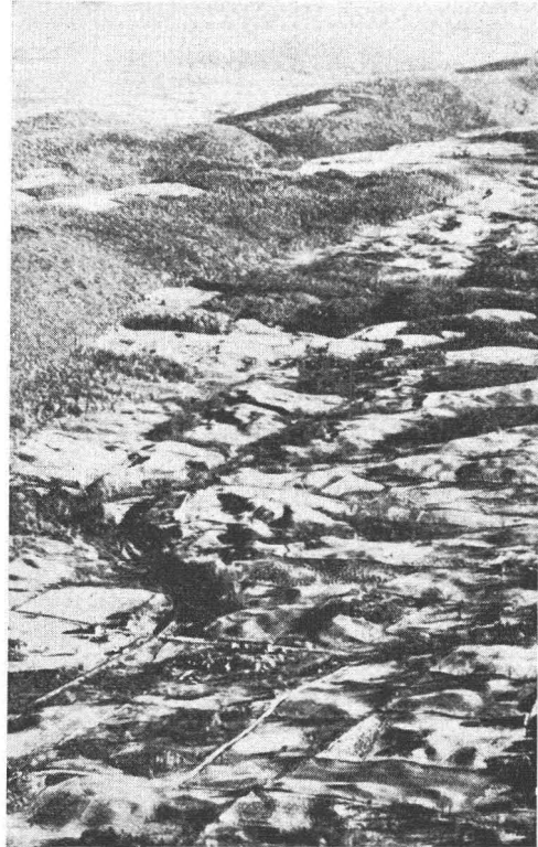
FIG. 1. Two adjacent, unlike land forms are shown in this aerial oblique. The numerous low hills in the central portion of the picture make up a group of morainic hills (one glacial land form). The massive ridges (upper left) are of hard shale. Rock cuts and drainage are major items in road construction in this land form, while items of frost heave, soft subgrades, swamps and earth excavation are important in the moraine.
