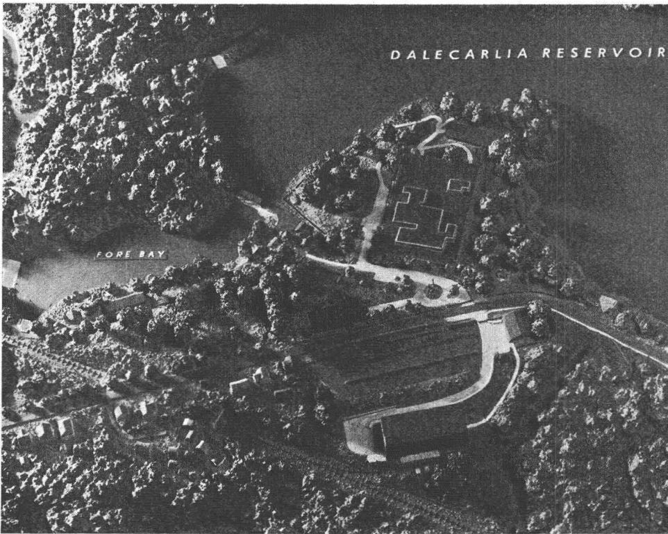
FIG. 4. This photograph illustrates the assault type model prepared for specific targets. It is a view of the 1:2,000 reproducible sponge rubber model of the Army Map Service as prepared by that Agency.
