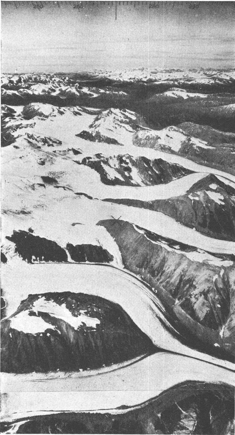
FIG. 9. Portion of a tri-camera composite, Eagle V cameras, 5×5 inch negatives, 3¼-inch Ross Wide Angle Survey Lens: From original 9×9 inch enlarged prints. Taken vicinity Bowser Lake, B.C. approx. 129°50'W, 56°35'N, in connection with an aerial reconnaissance of the "A" route from Hazelton, B.C., to Alaska. Oblique is directed northwesterly toward Unuk, Iskut, and Stikine Rivers. Note the striking evidence of the "recession" of glaciers in these views.
