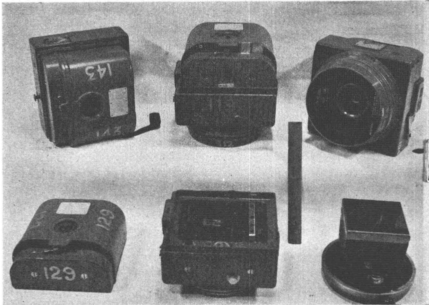
FIG. 3. Eagle V Air Camera with 3\frac{1}{4} -inch F/5.5 Ross Wide Angle Survey Lens.
