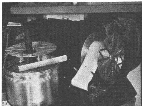
FIG. 8. Spiral Developing Outfit for 5½-inch film 60 feet in length.
