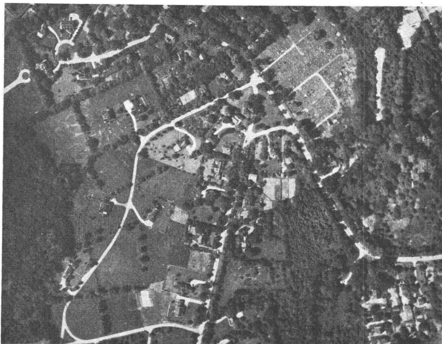
FIG. 7. Mapping run at 3000 feet 1/125 of a second—minus blue—45 MPH—3 prism.
