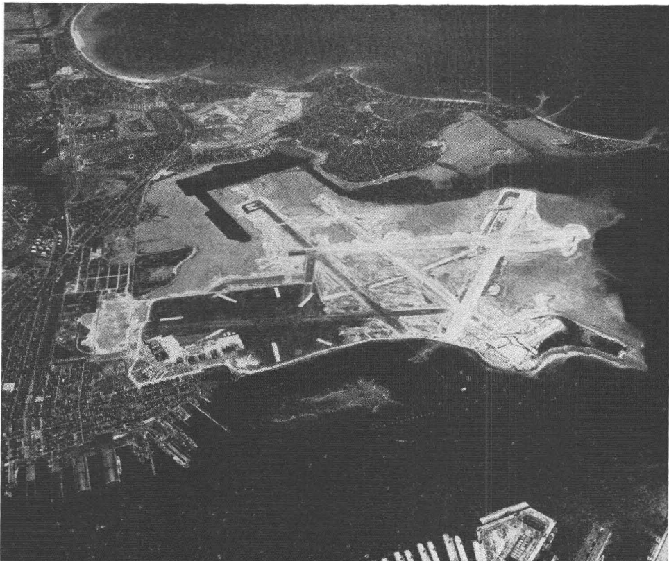
FIG. 2. An oblique has no common scale. The runways on the airport are approximately the same length, although measurements on the picture would not indicate this.—Mass. Dept. Public Works Photo.
