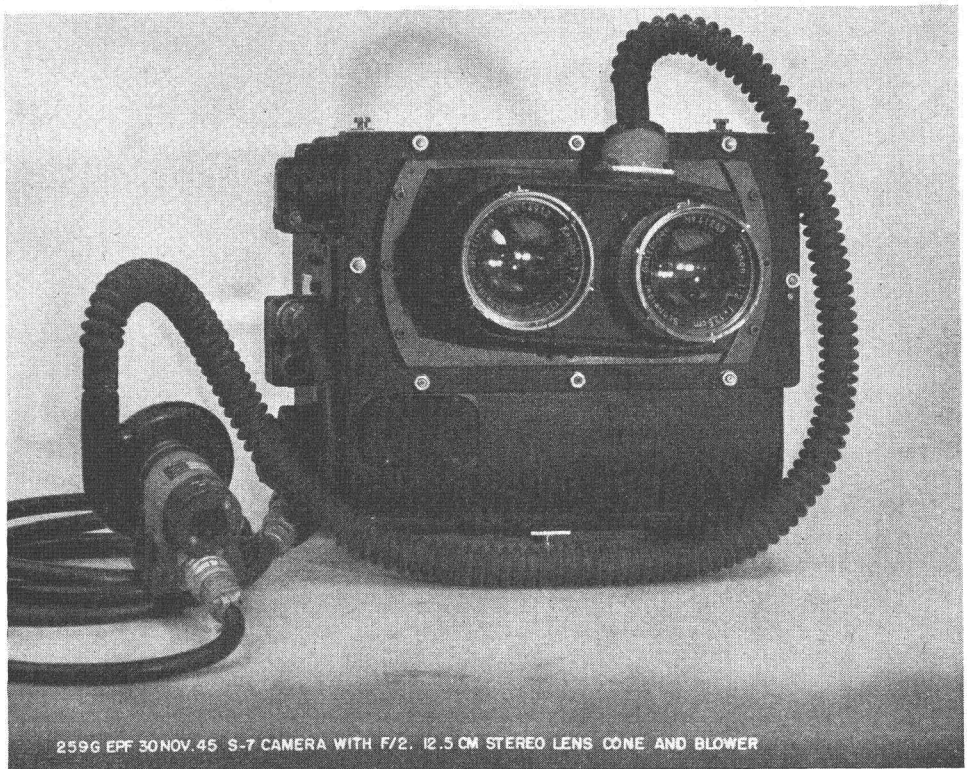
FIG. 21. Type S-7 Camera with Stereo Lens Cone.
