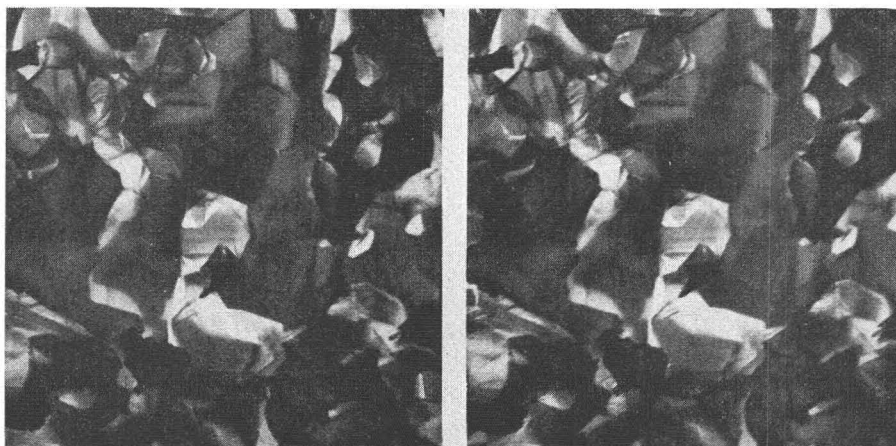
FIG. 9. Ni-Mn-O flake surface after heating 120 hours at 950°C. Mounted so as to give a view from inside the surface. "Shrouds" indicate presence of large inter-granular pores, relatively few in number.
