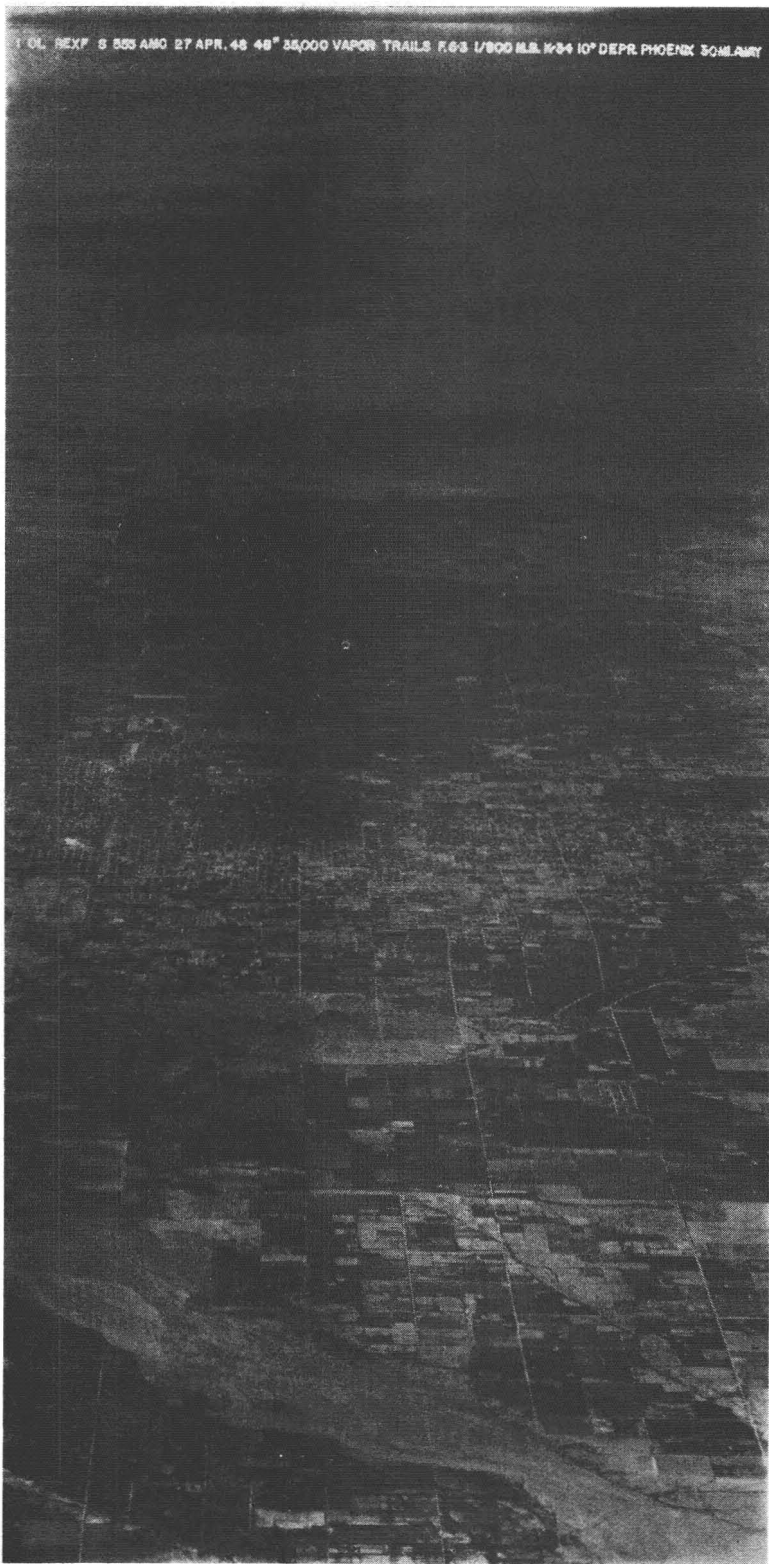
FIG. 6. A high altitude oblique photograph. Data: 48" f/6.3 lens, 35,000' altitude. Depression angle about 12°. Phoenix, in the center area of the photograph, is about 35 miles from the nadir point.
