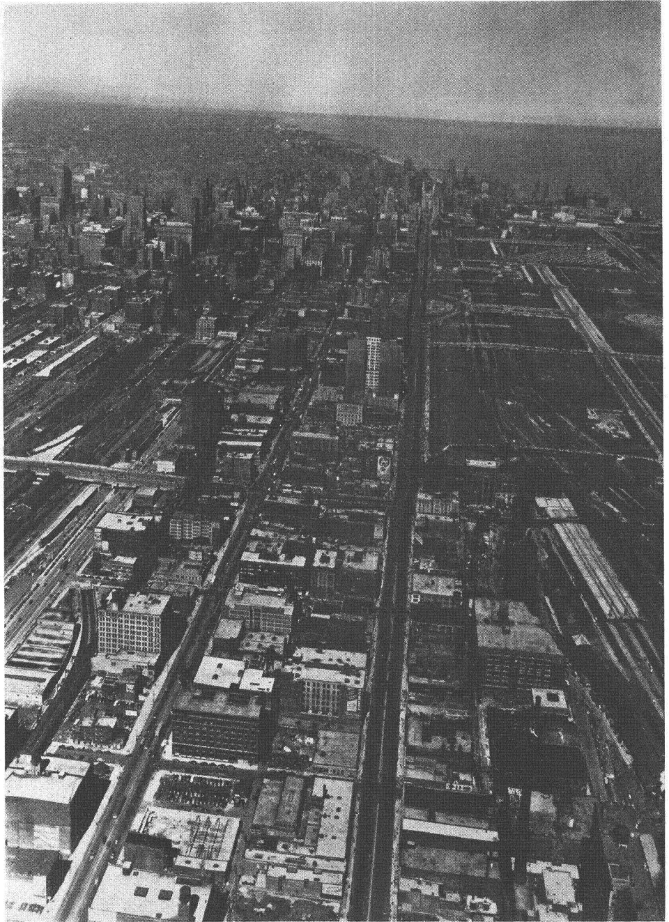
FIG. 12. Low altitude oblique photograph of Chicago. Camera used was K-27 (12" f/6.3 lens on 9"×18" format). Note the perspective effects, especially prominent in wide angle photographs.
