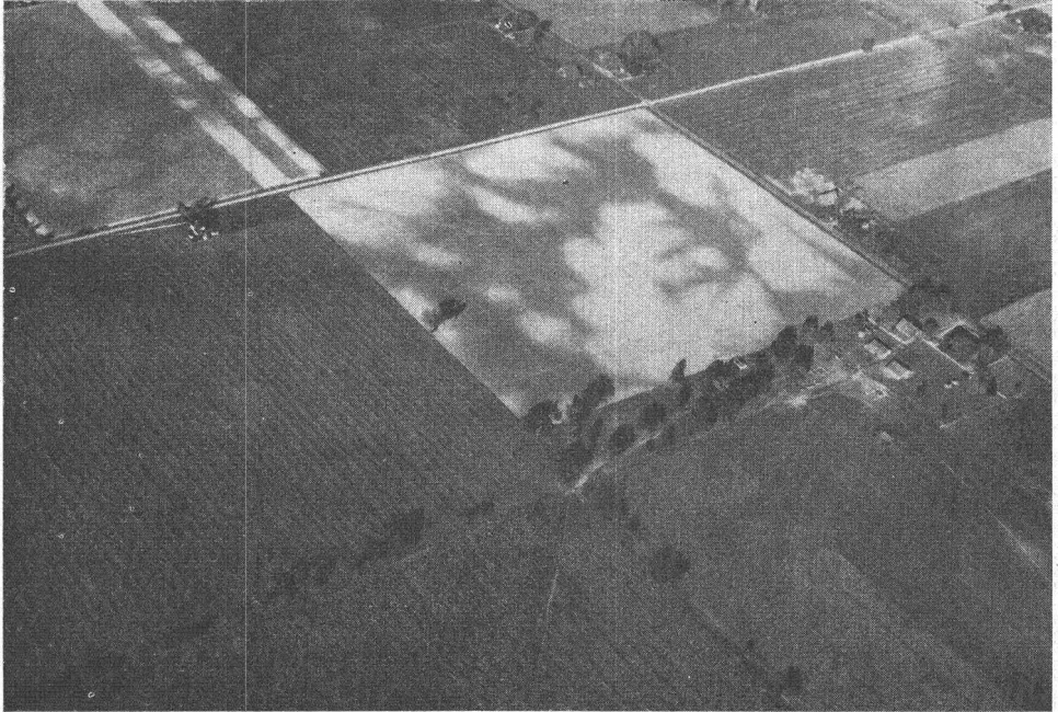
FIG. 15. Low altitude oblique airphoto of a Wisconsin glacial drift area. Tipton County, Indiana. The Brookston-Crosby soil pattern is easily identified even though the field has a cover crop. Faint near-white lines in some of the dark areas show a tendency toward gully development.
