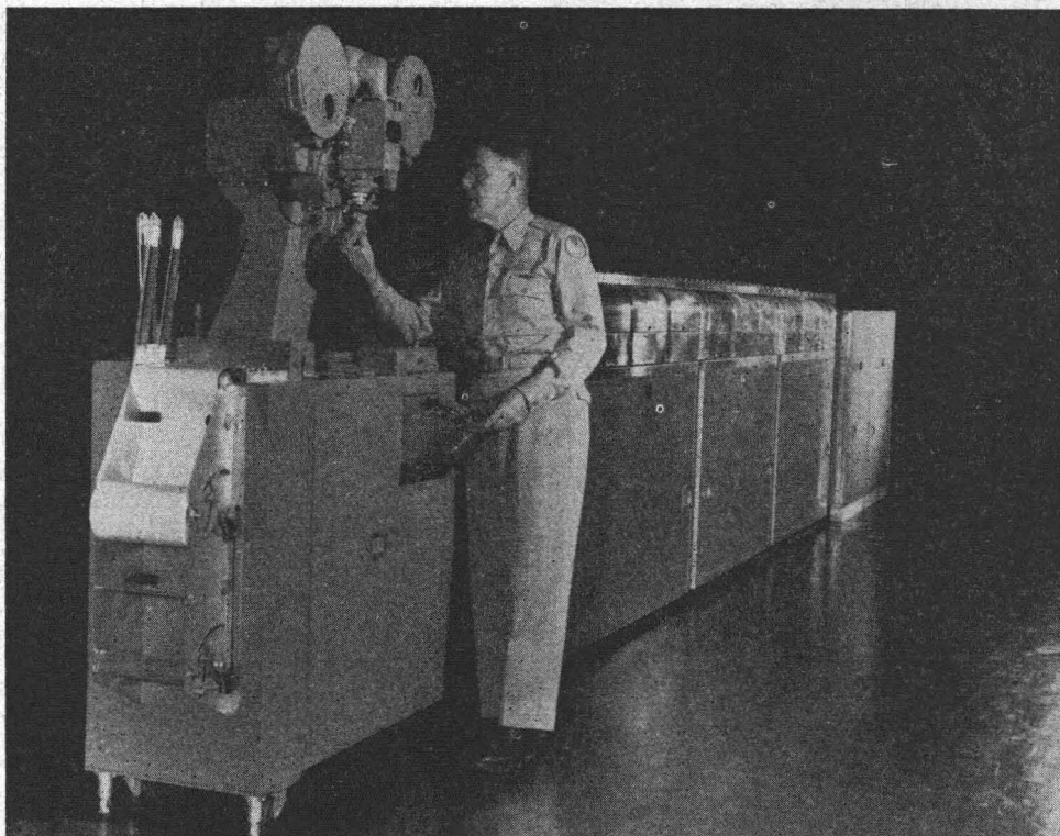
FIG. 1. Col. G. W. Goddard sets lens mechanism in photographic multiprocessor for negatives and prints.
