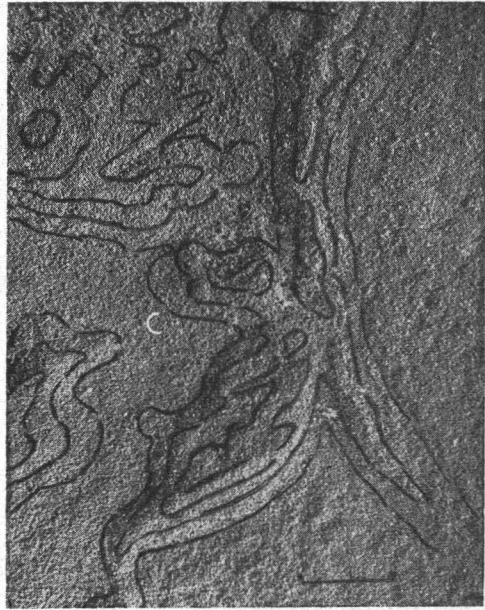
FIG. 3. A photograph of a mountainous region with rough form-lines sketched by hand under a mirror stereoscope. The black rod in this and the other photographs indicates a length of 800 m. Photo K.L.M. Copyright C.B.L.
