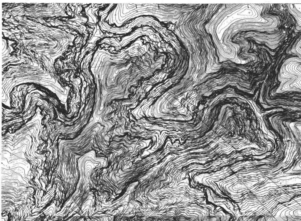
FIG. 5. A part of the Presidio River Survey for the location of the railroad between Durango and Mazatlan. Extremely difficult terrain full of inaccessible cliffs and tremendous differences in elevations will be noted. The Wild A-5 was used with 1/2,000 scale, 2 meter contours and an average flight altitude of 8,000 feet above the ground. A terrestrial survey of the area could have been made only with a tremendous amount of survey parties and would have necessitated great mountain climbing ability; the time of the job undoubtedly would have been several times longer.
